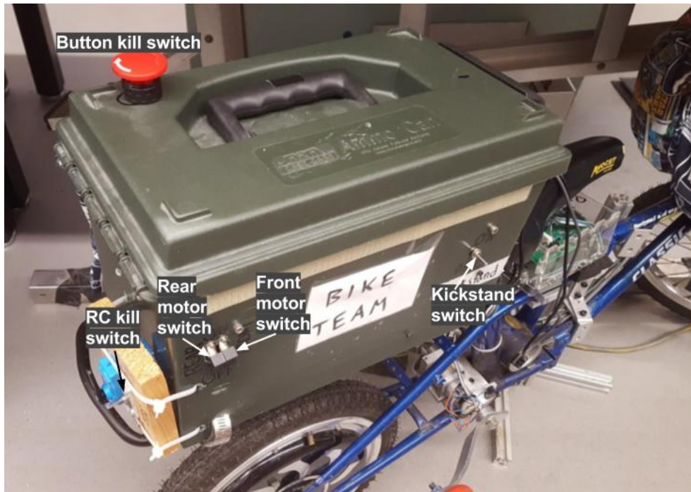
Figure 3.3: Drawing of Switches on Outside of Box
