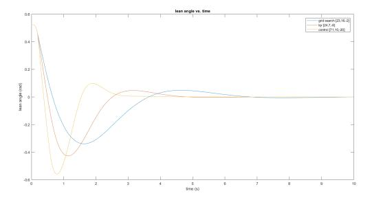
Figure 1: lean angle vs. time for 3 controllers
