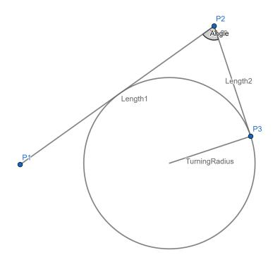
After this, if any part of the curve had a radius of curvature<sup>2</sup> smaller than the minimum turning radius of the bike, the Bezier-defining points were spread further apart to create a smoother curve.
