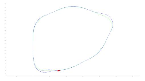
Figure 5: Green: result of path smoothing. Blue: path of bike
