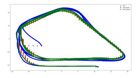
**Figure 2:** Position estimates using three different systems: red is GPS, blue is old (single-filter) Kalman, green is new (dual-filter) Kalman. The test included walking, 4 times, around a path on the engineering quad. The old (single) Kalman filter (blue) overshoots the top turn more than the new (double) Kalman filer (green).
