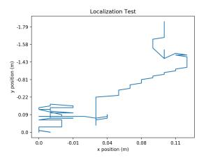
From our positional tracking, we get a timestamp, a 3D displacement vector, and angles for heading. We tested the tracking by plotting data collected while moving the buck against time. RTAB-Map and the Zed SDK also come with built in visualizers that use Rviz, so we can see how the data changes in real time.
