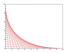
Figure 4: An example quadratic Bezier curve, defined with the points (0, 10), (0, 0), and (10, 0).
