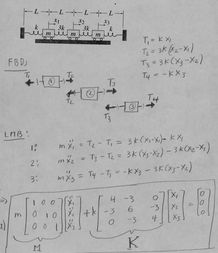
By symmetry, one normal made is!  $\begin{vmatrix} x_1 \\ x_2 \\ x_3 \end{vmatrix} = x_6 \begin{vmatrix} 1 \\ 0 \\ -1 \end{vmatrix} \sin(\omega t)$ Middle mass is still, so the side mosses see this Jun 10-11 & Jun 10-11 => 1 4k x=0 => X= Xo sinat LV44m = 2VEm (b) Mode shape = [], frequency w= 2/m/
