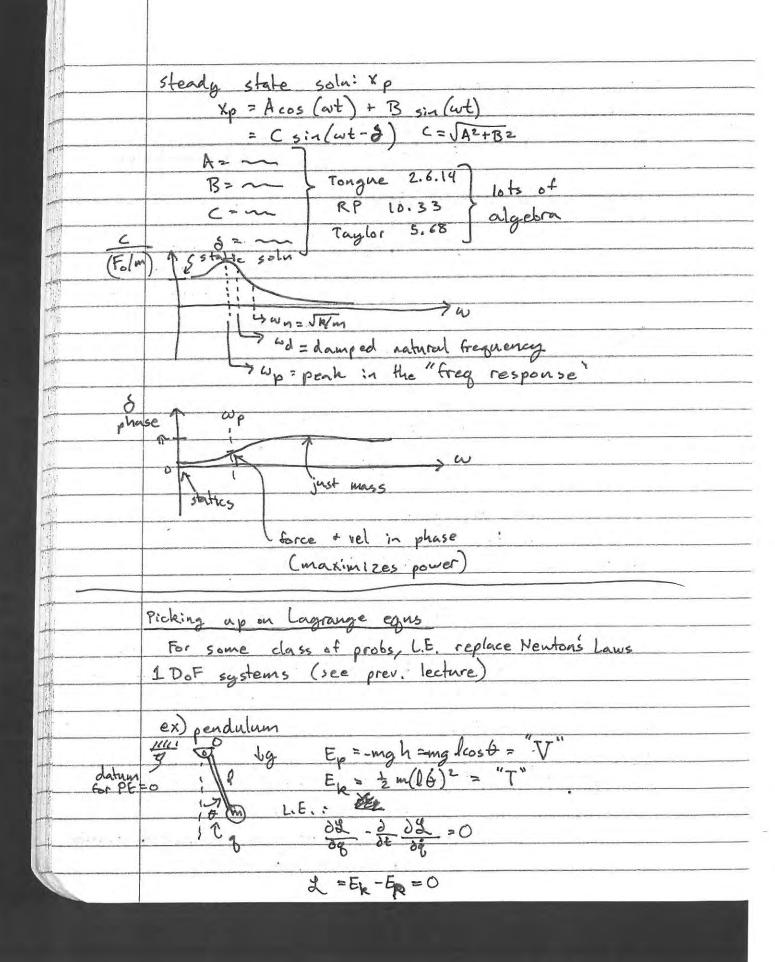
L.E.: 38 - 1 38 =0 2=Ex-Ep= 2m2/202 + mg/cost => (-mg l sin d) - d (m 3/26) =0 - rglsind - wl2 0 = 0 0 + 7 sind = 0 The pendulum egn 0=0 Near equilibrium D << 1 D + \$ D = 0 linearized pend egn
