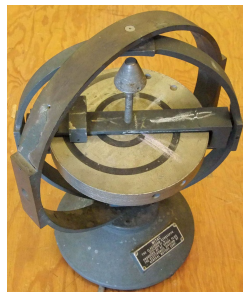
Figure 4.1: A demonstration gyroscope mounted on gymbals. The disk with the spiral marked on it is free to rotate in three dimensions because it is free to rotate about the three gymbal bearings: one with a vertical axis, one with a horizontal axis and one with an axis normal to the disk.
