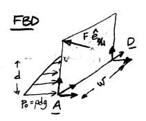
The hydrostatic pressure Po = pgd acts across the entire width of the door and so is equivalent to a loading q = pgdw
