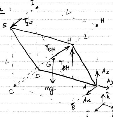
Like problem 4.87 in HW2, part b) let us try finding as many unknown reactions as possible by using balance of moment about an arbitrary axis.
