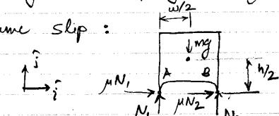
$$\left. \begin{array}{l} \{LMB\} \cdot \hat{j} \Rightarrow N_r + N_f = mg \\ \{LMB\} \cdot \hat{i} \Rightarrow \mu N_r + \mu N_f = ma \end{array} \right\} \Rightarrow a = \mu g$$
