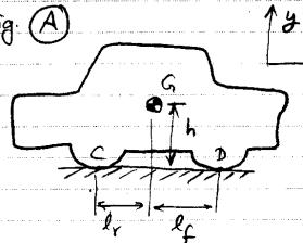
To know the deceleration, reaction forces for different case of skidding.
