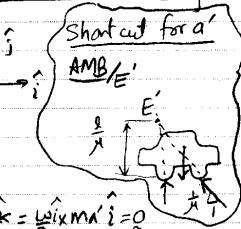
$$\{AMB\}_{A'} : (-\mu N_f h - mg\frac{\omega}{2} + N_f \omega) \hat{k} = \frac{\omega i \times ma}{2} \hat{i} = 0$$
