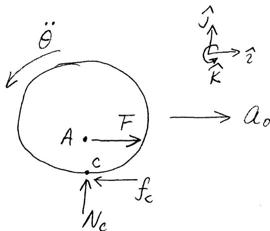
Kinematic constraint:  $\ddot{\theta} r_2 = -a_0$
