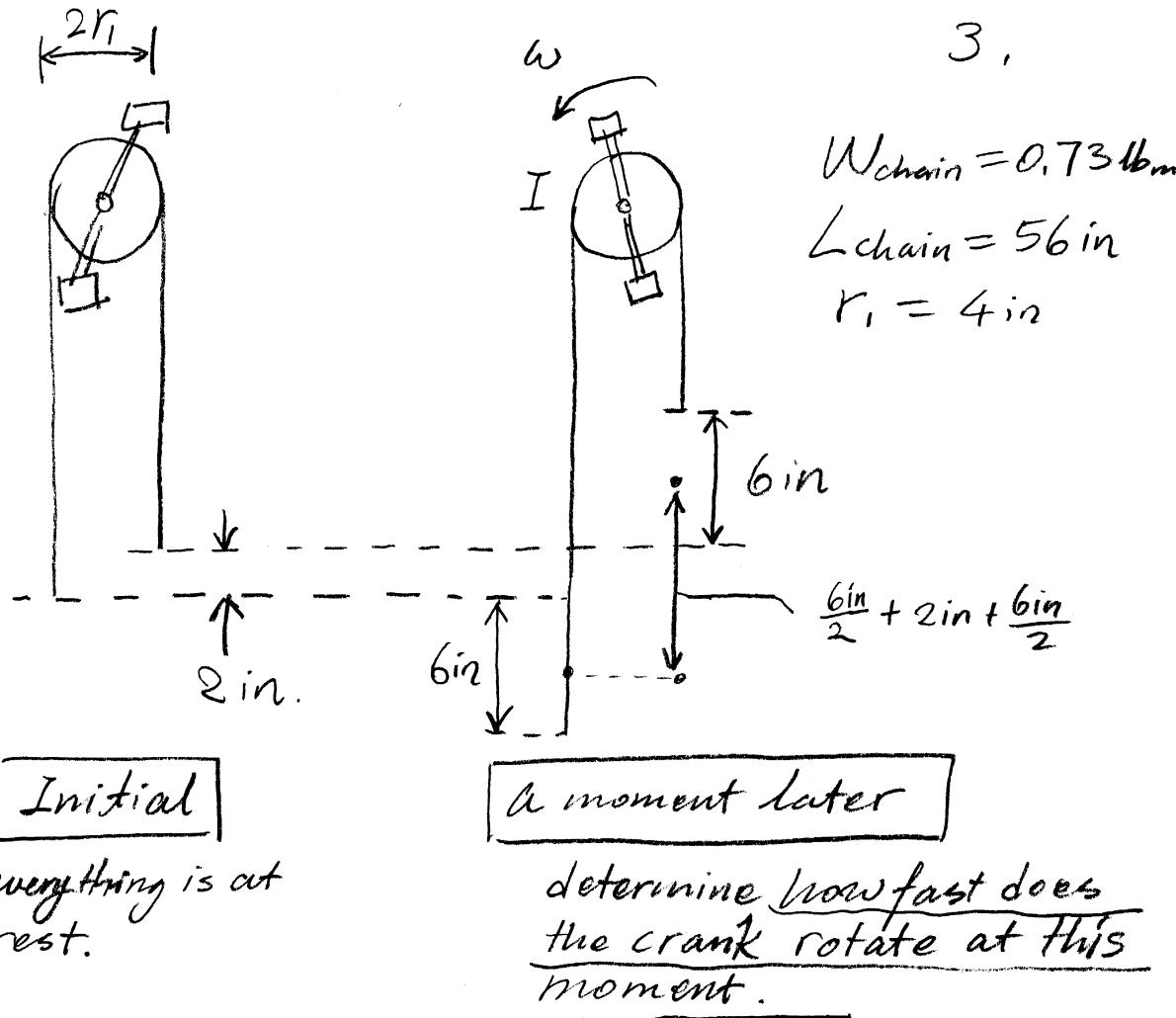
Solution The whole chain moves at speed of  $|w r_1|$ . Thus,
