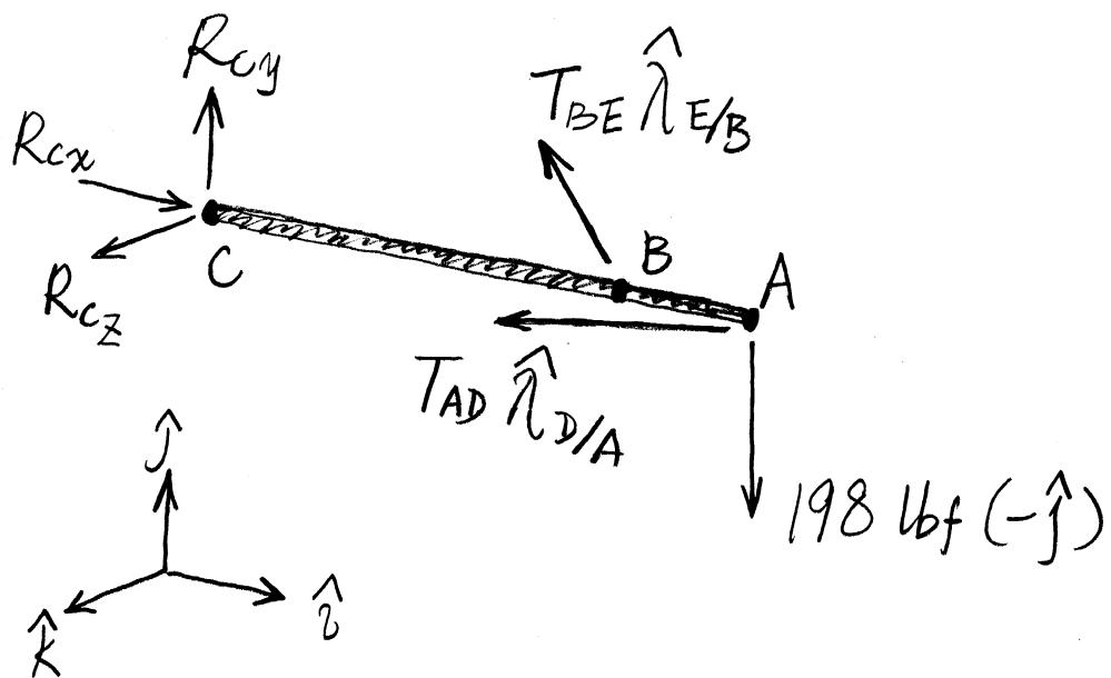
Solution Our goal is to find tension in cable BE only. Thus, we should observe that the reaction force at C (i.e.,  $R_{Cx}\hat{i} + R_{Cy}\hat{j} + R_{Cz}\hat{k}$ ) and the force on the boom from cable AD (i.e.,  $T_{AD}\hat{\lambda}_{D/A}$ ) both pass through line DC. Thus, the moment produced by them about axis  $\frac{\vec{r}_{DC}}{\|\vec{r}_{DC}\|}$  is ZERO!
