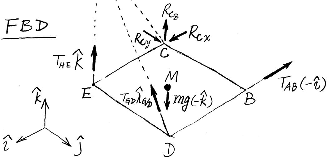
Solution Our goal is to find the tension in cable AB only. Thus, we should observe that the reaction force at C (i.e.,  $R_{Cx}\hat{i} + R_{Cy}\hat{j} + R_{Cz}\hat{k}$ ),  $\vec{R}_{EC}$  (the force on the shelf from cable HE), and  $\vec{T}_{GD}\hat{l}_{GD}$  (the force on the shelf from cable GD), all of them pass through line GC.
