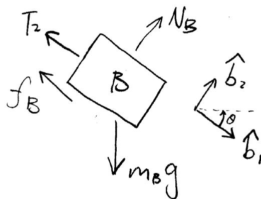
Notes: ① at the critical equilibrium state, A tends to move to the right while B tends to move down along the inclined surface although both A & B are still at rest. At this state,  $f_A = N_A \mu_s$  and  $f_B = N_B \mu_s$ . Their directions are opposite to the directions A and B tend to move.
