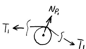
$\Rightarrow$  the tensions in the rope on both sides of Pulley  $P_1$  are the same, i.e., both are  $T_1$  (this is also true for part c.)
