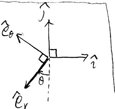
$$\begin{aligned} \hat{j} \cdot \hat{e}_\theta &= \omega s(180^\circ - 90^\circ - \theta), & \hat{i} \cdot \hat{e}_\theta &= \cos[90^\circ + (180^\circ - 90^\circ - \theta)] \\ &= \sin \theta & &= -\cos \theta \end{aligned}$$
