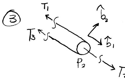
Pulley  $P_2$  is massless, round, and frictionless
