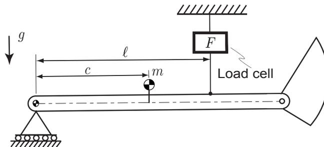
Figure 23: **Experiment to measure the first mass moment  $c \cdot m$ .** The robot is hinged at the hip joint and held such that the leg axis is perpendicular to gravity. Balance of moments about the hip hinge gives  $mc = F\ell$ .
