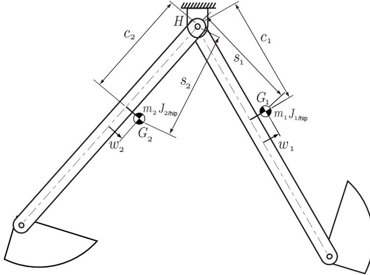
Figure 22: **Dynamic balance of the legs.** The two legs of the robot are dynamically symmetrical (‘balanced’) if they have the same distances between the hip and ankle hinges, the same foot shapes and have 3 matching inertial properties. The two masses do not have to be the same, however.
