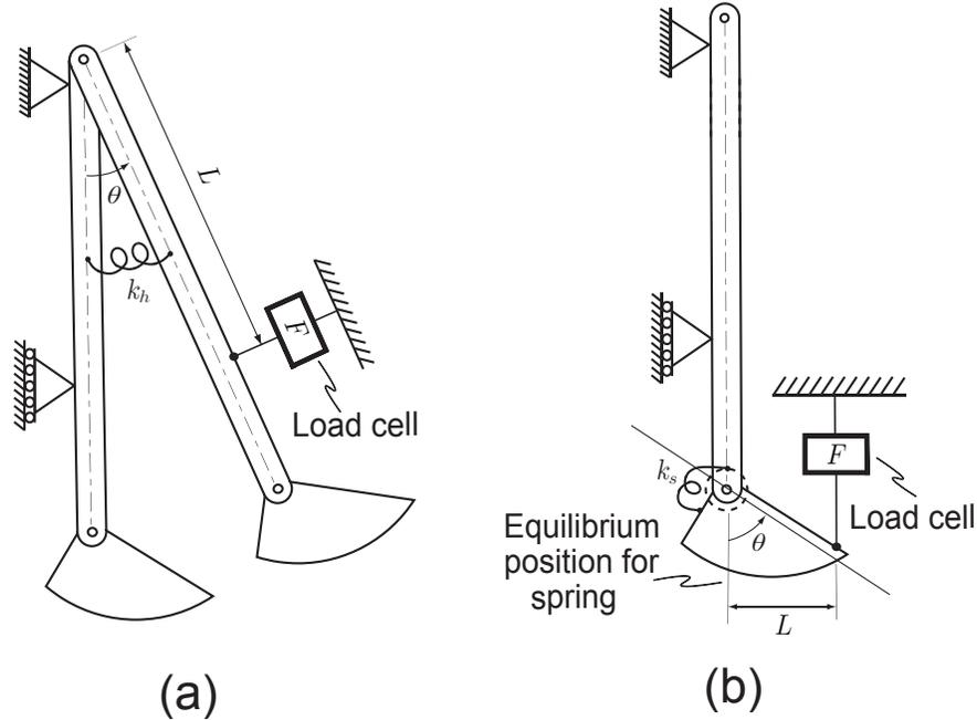
Figure 25: **Measuring the spring constants.** **a)** The hip spring stiffness (see figure 6 on page 12 and related text) is determined by measuring the force to deflect the leg a given angle. **b)** The ankle spring constants (the elasticities of the cable drive, see figure 3 on page 9 and related text) are measured by locking the ankle motors and measuring the force to deflect the ankles.
