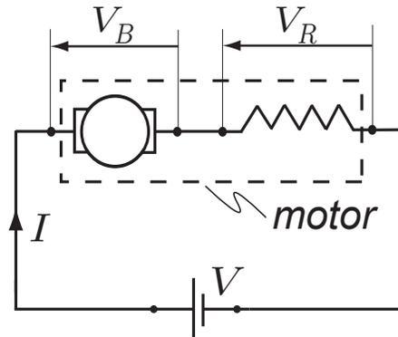
Figure 27: **Schematic of DC motor connected to a DC voltage source.** The DC motor consists of rotating part called the rotor and a resistive part. The sum of voltage drop across the rotor ( $V_B$ ) and resistive part ( $V_R$ ) equals the total voltage supplied by the DC source  $V$ . The current flowing in the circuit is  $I$ .
