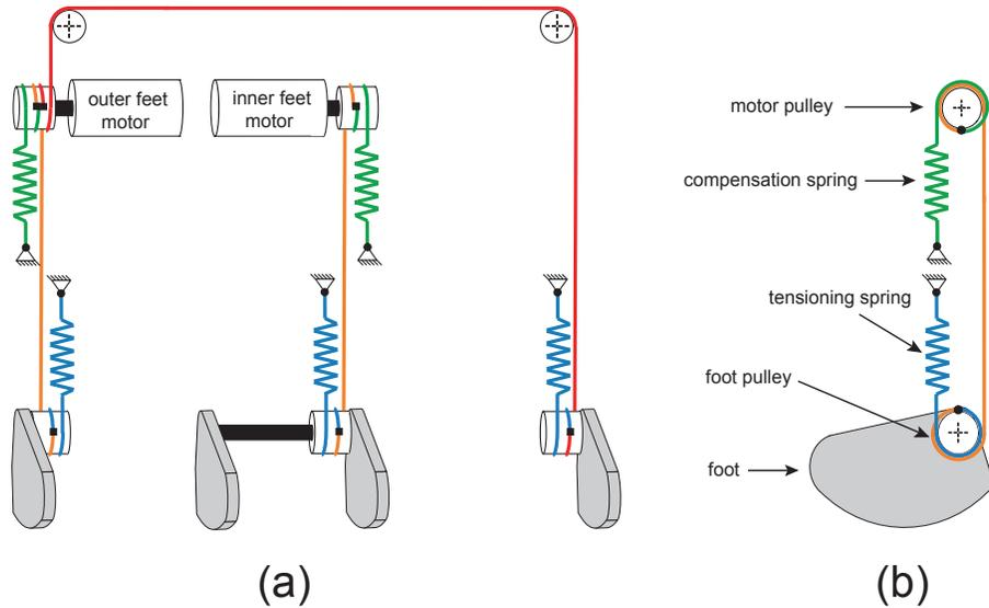
Figure 3: **Ankle actuation.** (a) Perspective schematic, (b) Side schematic of one leg. One motor controls the inner ankles and one controls the outer ankles. For each leg pair ankle extension (e.g. push-off) is powered by a single cable and retraction (for foot ground clearance) is powered by a return spring. Another return spring on the motor prevents cable slack when the motor is off, and also balances out the force of the ankle return spring so that the motor doesn't have to.
