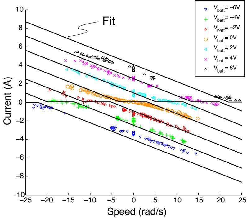
Figure 29: **Curve-fitting for motor torque constant.** Motor torque constant  $K = 0.018 \text{ V s/rad}$  was curve-fitted from equation ?? using motor current  $I$ , output shaft speed  $\omega$  and DC voltage  $V$  data obtained from the cantilever set-up. In equation ?? we used gear ratio  $G = 14$  as per manufacturer's specification. Constants  $R = 1.3 \Omega$  and  $V_c = 0.7 \text{ V}$  were obtained in an earlier experiment (see figure 28).
