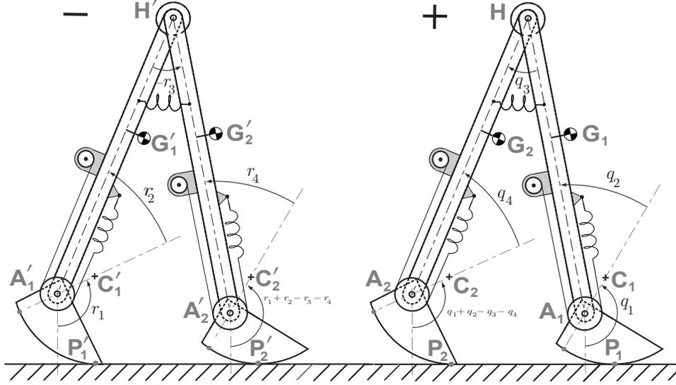
Figure 18: **Angle swap for heel-strike derivations.** The instant just before heel-strike is denoted by  $-$  and the instant just after heel-strike by  $+$ . We swap the names of the legs during heel-strike as shown. To simplify notation the angles are named  $r_i$  before collision and  $q_i$  after collision., where  $i$  is the joint number.
