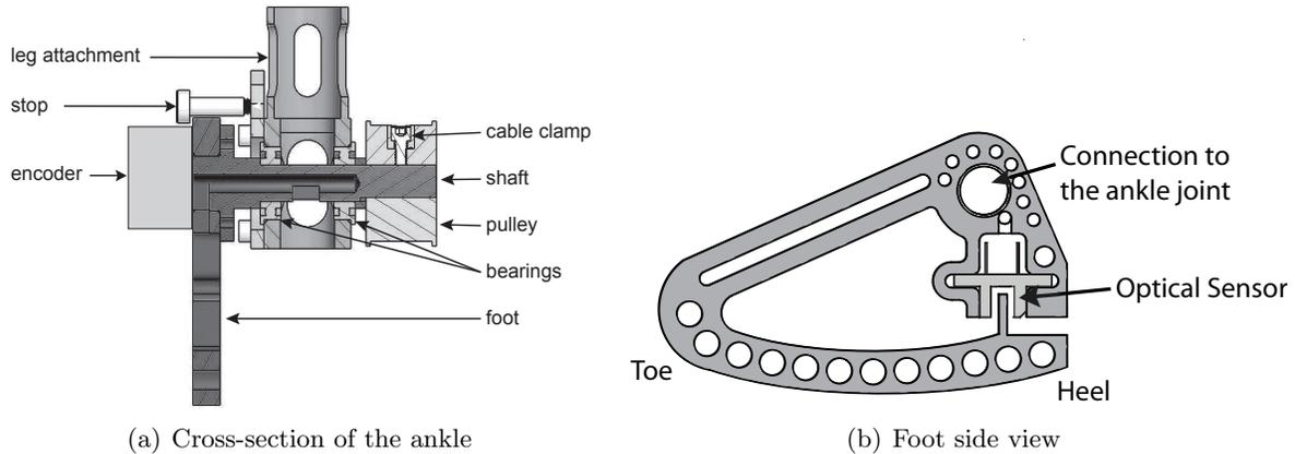
Figure 4: **Ankle and foot.** **a)** Front view of a cross-section of the foot-ankle assembly, **b)** Side view of the foot. The top of the foot hits the stop when the top of the foot is approximately vertical. The ‘stop’ includes a spring-loaded electrical contact, thus acting as both a mechanical stop and an electrical limit switch.
