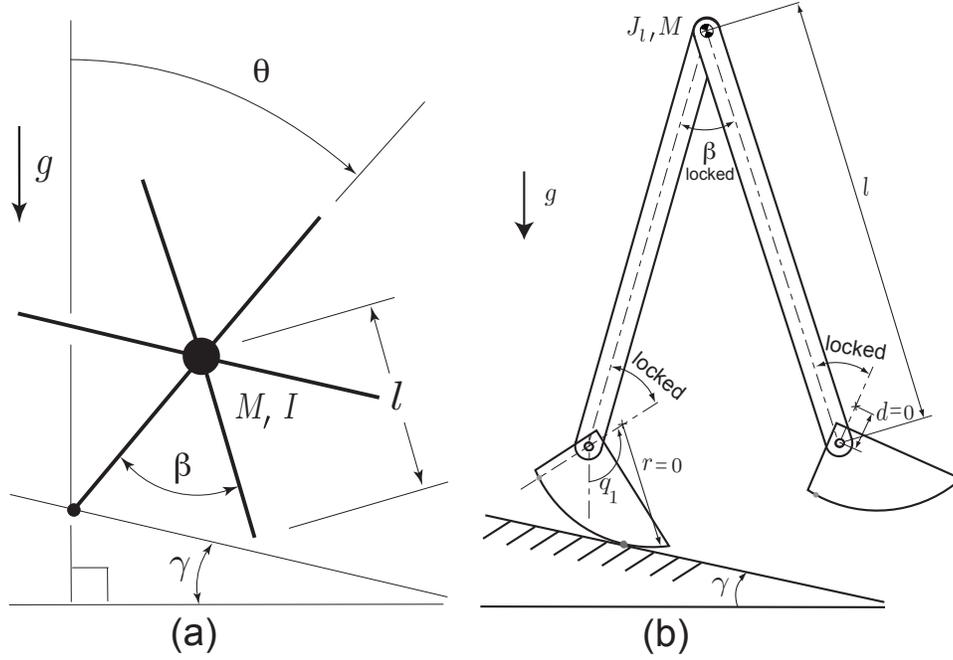
Figure 20: **2-D rimless wheel.** (a) 2-D rimless wheel analyzed by Coleman. (figure source: Coleman's PhD thesis [1]), (b) Ranger model simplified to a rimless wheel; The hip angle and ankle angles are locked and the centers of mass of the leg are put at the hip.
