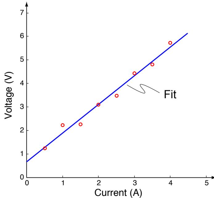
Figure 28: **Curve-fitting for contact voltage and terminal resistance.** Least squares curve-fitting voltage and current data for a stalled motor gives a terminal resistance  $R = 1.3 \Omega$  (slope) and contact voltage drop  $V_c = 0.7 V$  (y-intercept).
