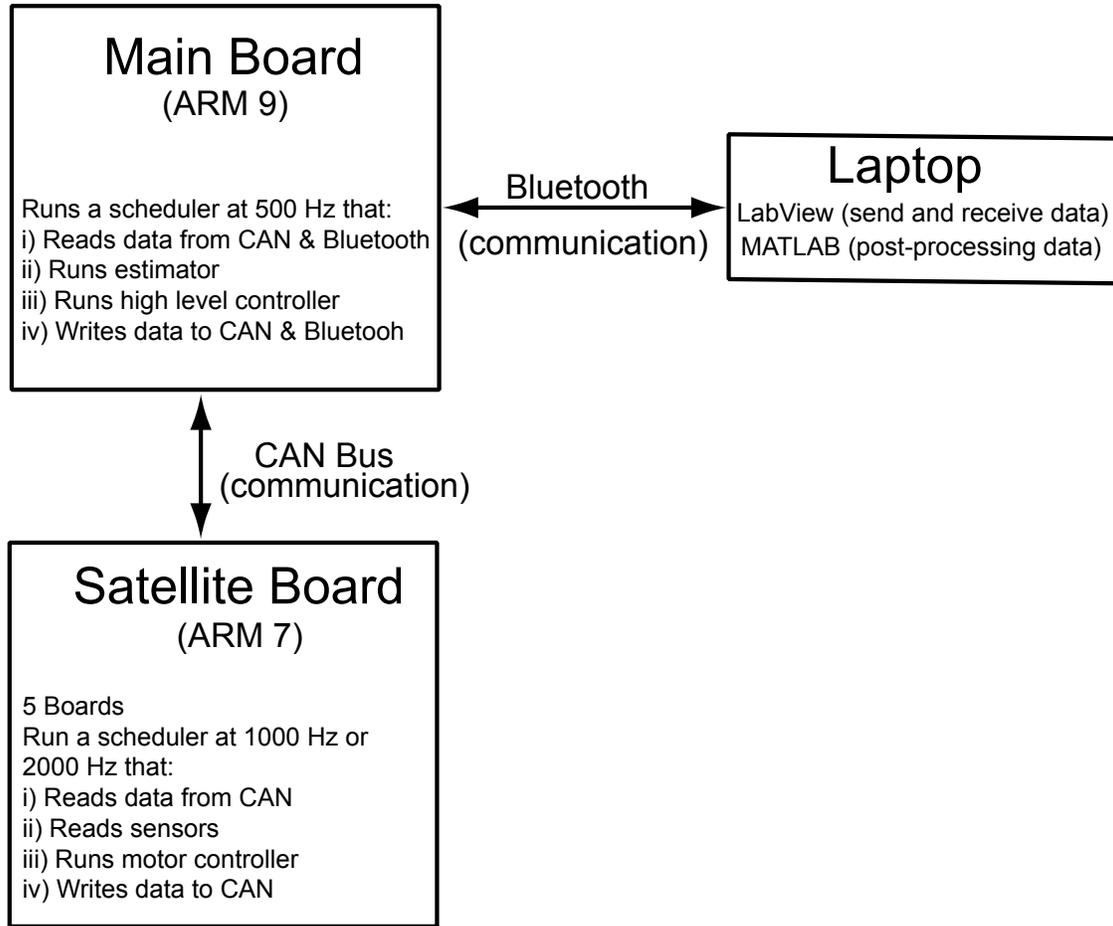
Figure 8: **Overall electronics architecture.** An ARM 9 ‘main brain’ communicates with 6 ARM 7 satellite processors via a CAN network. Data collection and tuning use a Bluetooth wireless data link. Not shown is the hobby radio control used for steering.
