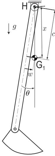
Figure 24: **Experiment to measure the fore-aft offset of the COM.** The robot is hinged at its hip joint  $H$  and held in the vertical plane. In equilibrium the center of mass of the leg  $G_1$  is directly below the hinge point  $H$ . The angle  $\theta$  can be measured.
