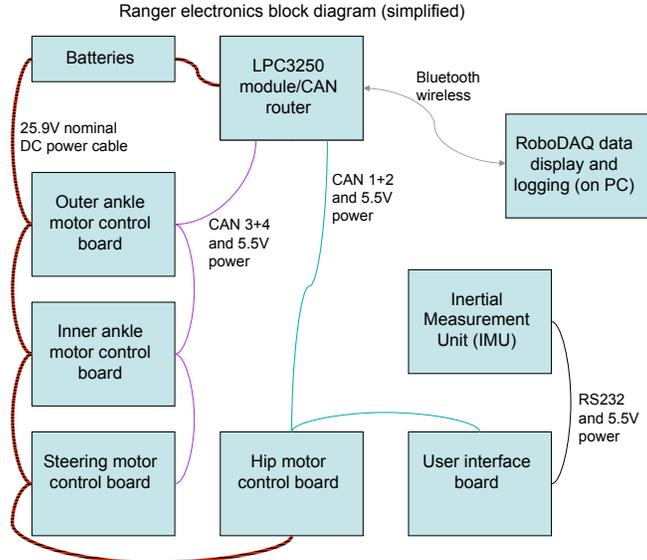
Figure 10: **Wiring between microprocessor boards.** Dark red is main power. Violet and light blue are CAN buses. The CAN router board is the port for information to and from the main brain (which is not shown).
