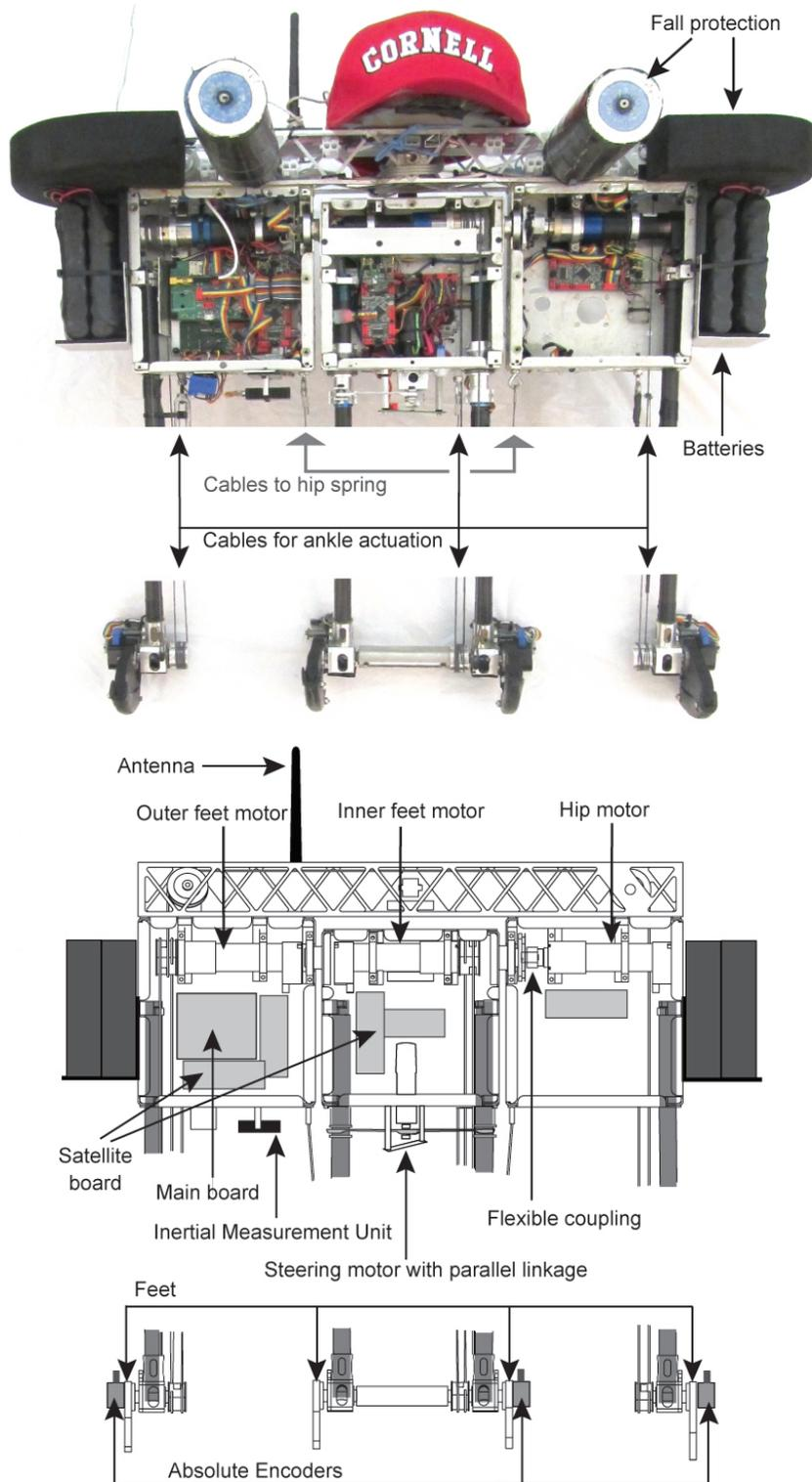
Figure 2: **Overall layout, front view.** In the photograph the boxes are open. The foam assemblies for fall protection ('eyes' and 'ears') serve no other purpose. The hat is only decorative. The main and satellite boards contain most of the electronics. More details are in the text and following illustrations.
