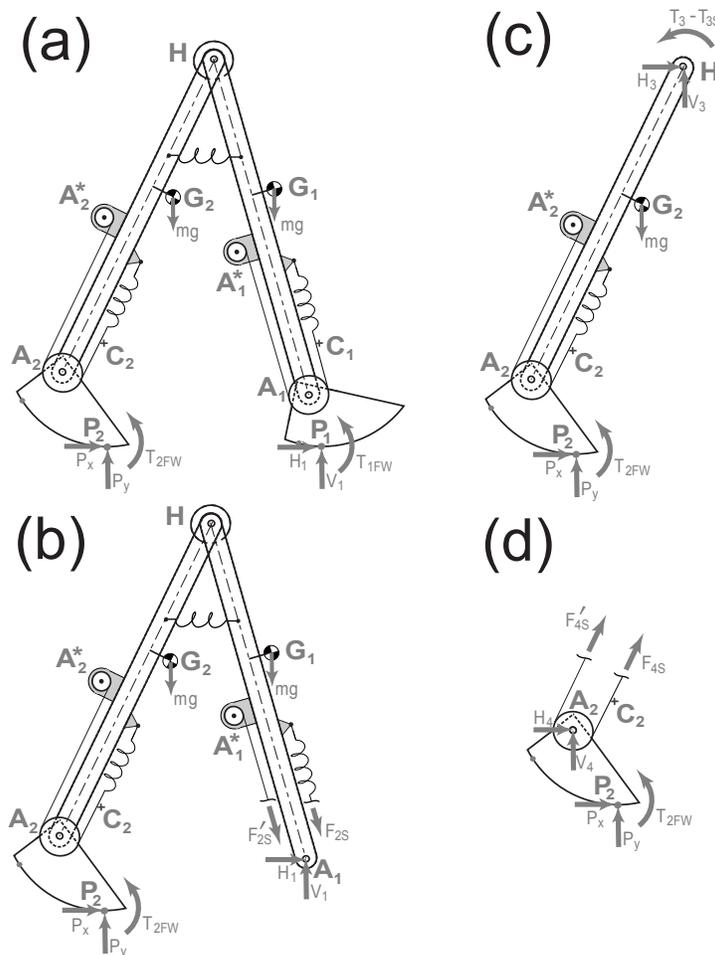
Figure 16: **Free Body Diagrams (FBD) to derive equations for double stance.** We have four free body diagrams. The arrows indicate all of the non-neglected forces and torques acting on each of the four systems.
