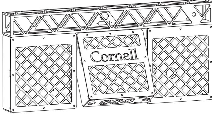
Figure 5: **Legs supporting structures (hips/thighs)**. Each outer leg has one closed aluminum box made from folded and welded sheet stock. The pair of inner legs has a similar closed box. The outer boxes are joined by a truss made from a hollow aluminum box beam with triangles machined out to reduce weight. The inner box is hinged to the outer boxes by the hip axle which runs parallel to, and below, the truss.
