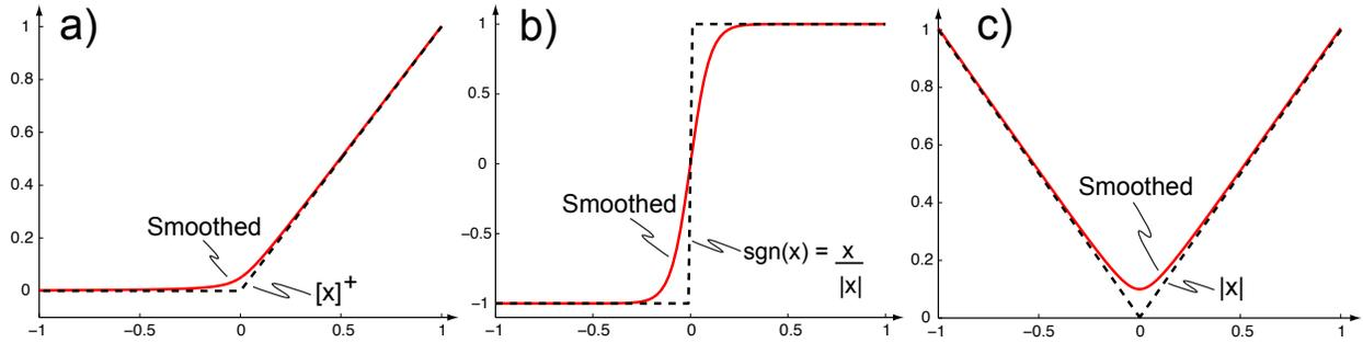
Figure 32: **Smoothings for discontinuous functions.** The smoothings for a unit ramp function, a step function and for the absolute value function (dotted black lines= function, solid red lines = our approximation).
