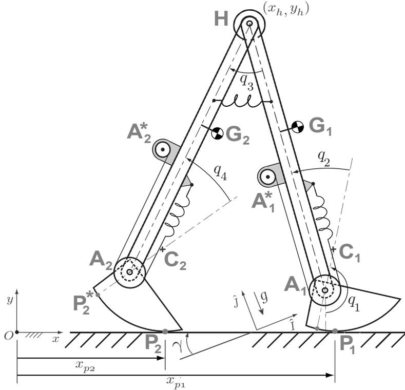
Figure 15: **Robot reference frames and degrees of freedom used in the derivation of the equations of motion.** The absolute angle made by the lead foot on the ground with the vertical is  $q_1$ . Joint angles are  $q_2, q_3$  and  $q_4$ . Hip motor angle is the same as hip joint angle  $q_3$ . Ankle motor angles associated with the joint  $A_1^*$  is  $q_{2m}$  and with joint  $A_2^*$  is  $q_{4m}$ .
