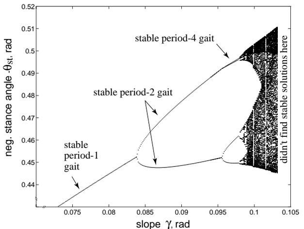
Figure 4: Period doubling route to chaos in *stable* kneed walking motions. The parameters are those of the zero-slope capable walker labeled (C) in figure 6.
