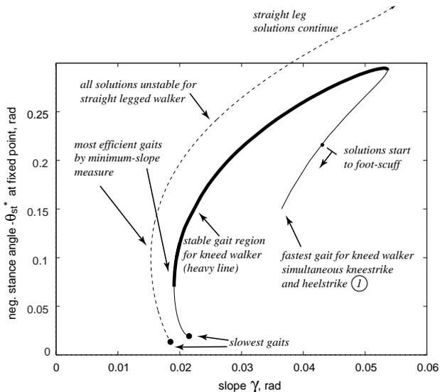
Figure 3: Calculated locus of solutions showing fixed points of stance angle as a function of slope for our physical kneed walking model (solid line) and for the same model but with the knees locked (dashed line). Each point on this graph is one periodic solution. The thick portion of the solid line denotes stable solutions for the kneed walker.
