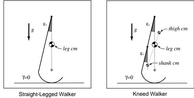
Figure 5: **Necessary conditions for near-zero slope walking.** The separations between the hips and the mass centers shown here are larger than those typical for our simulations. The necessary condition for elimination of first-order scuffing from knee flex is not shown.
